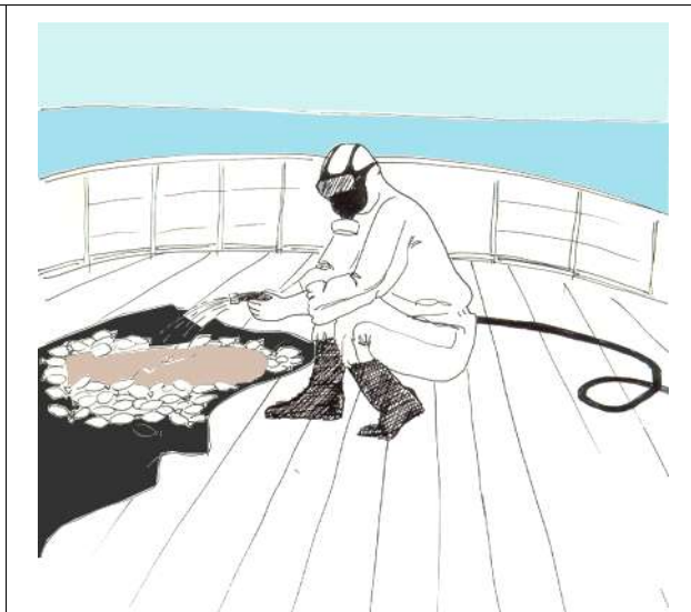
2. if fumes are emitted wear the protective clothing and keep the device wet by spraying it with a low pressure jet of water.
