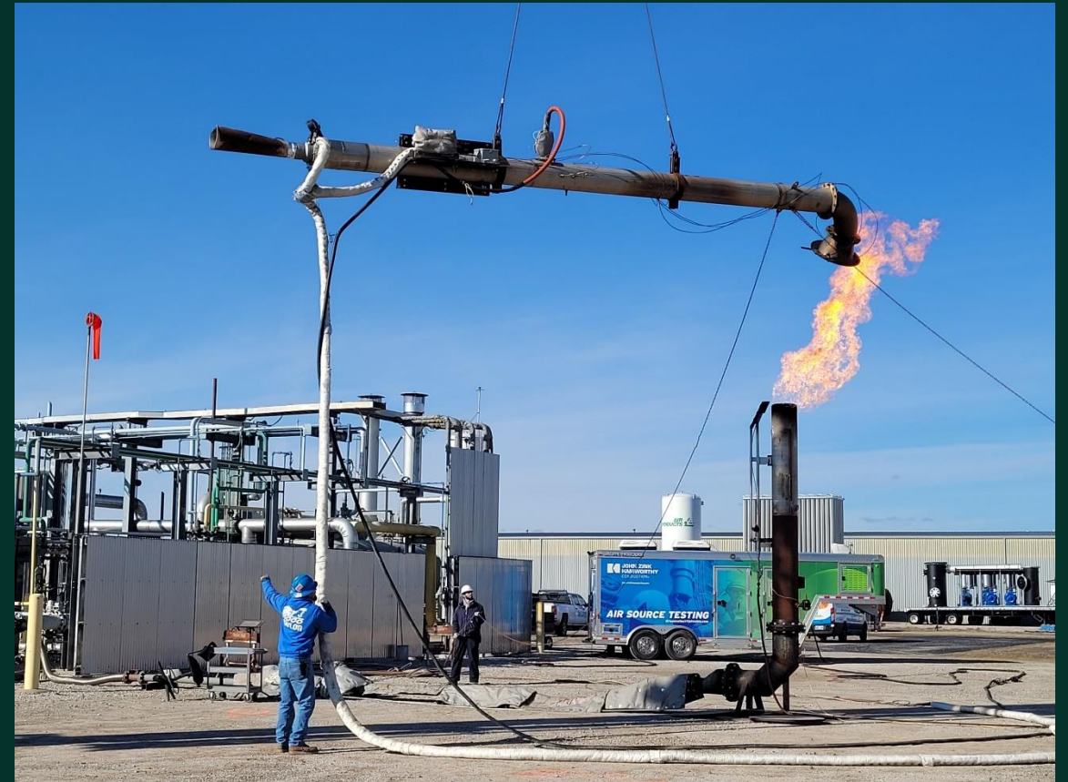
flare.IQ testing with extractive sampling in full swing
