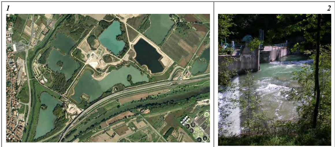
Figure 58 – Other structures (besides those defined for A1) that can cause an alteration of flows within a reach. (1) Retention basins; (2) discharge abstraction.
