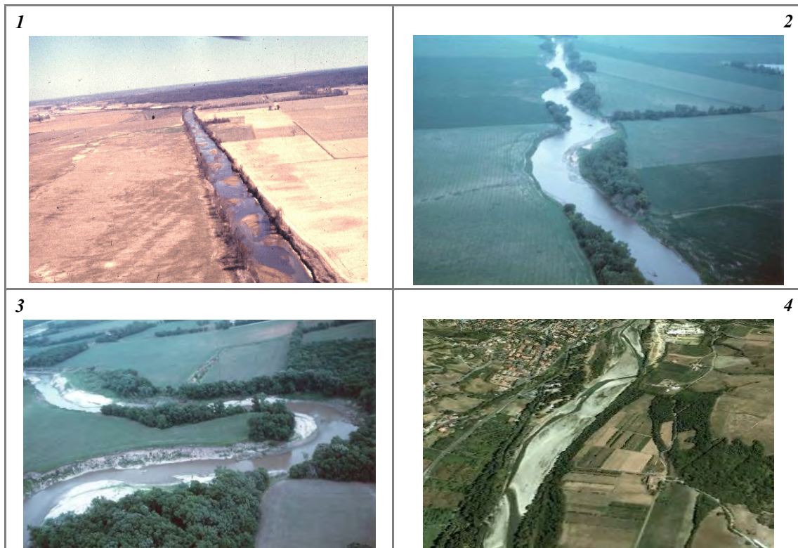
Figure 6 – Examples of morphologies of partly confined and unconfined channels. (1) Straight; (2) sinuous; (3) meandering; (4) sinuous with alternate bars.
