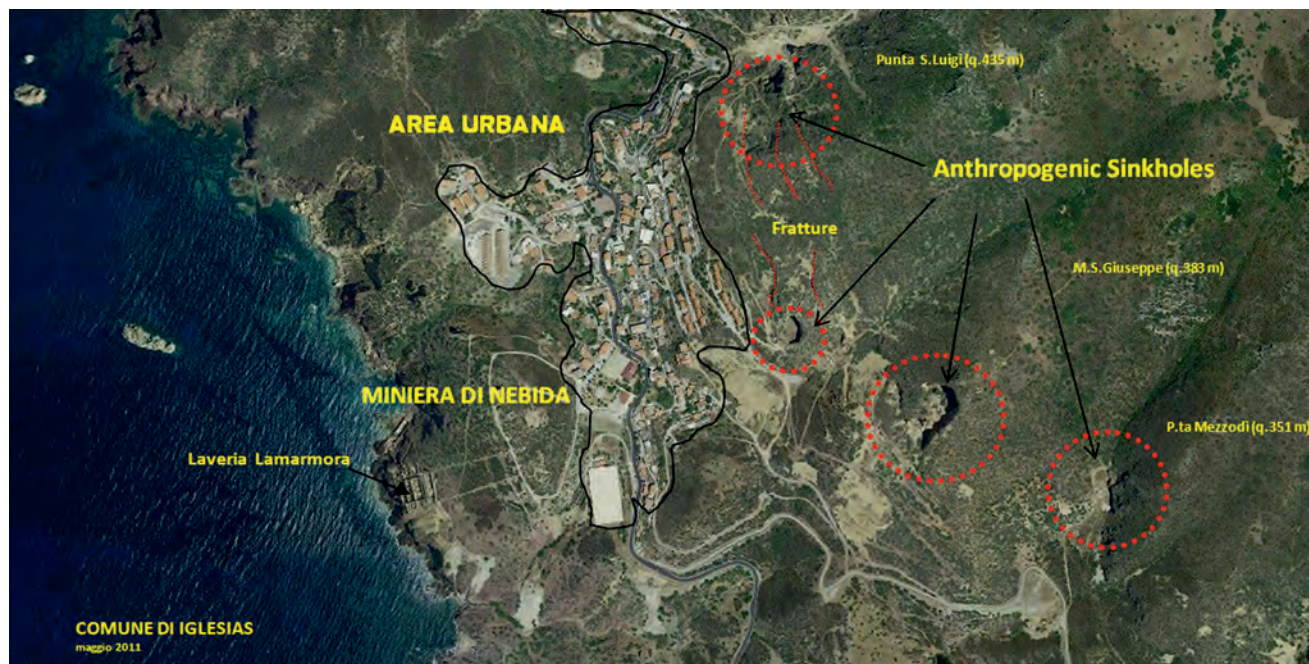
Fig. 8 – I sinkholes e le fratture localizzate a monte del borgo minerario di Nebida (comune di Iglesias - Sardegna sud occidentale). – The sinkholes and fractures located upstream of the mining village of Nebida (Municipality of Iglesias – South - Western Sardinia).
